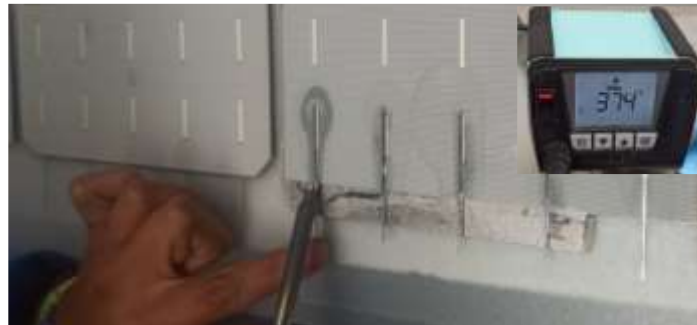
Figure 20 Joining process of monocrystalline cells by means of the soldering station
