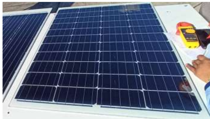
Figure 21 Assembled monocrystalline photovoltaic module (by welding)
